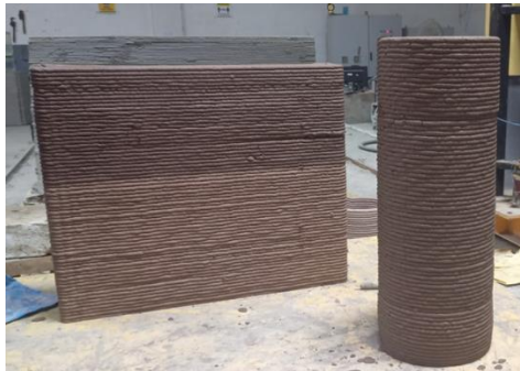
Figure 8: 3D printed elements using low carbon binder and high aggregate to cement ratio
