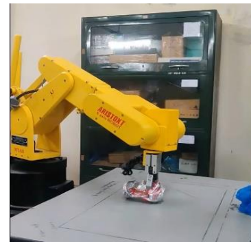
Figure 5: 6DOF industrial robot being trained to pick & place recyclable objects
